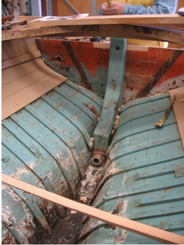
The bilge and motor bay before installation of the electric motor
