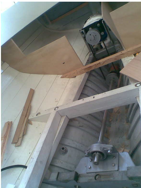
Electric motor and drive shaft
