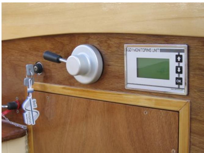
The display and throttle are built into the aft liner of the boat.
