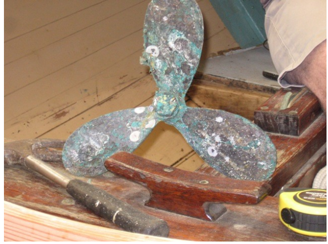
After a clean & polish the existing propeller can be retained with the new electric motor and will rev at 1600 RPM
