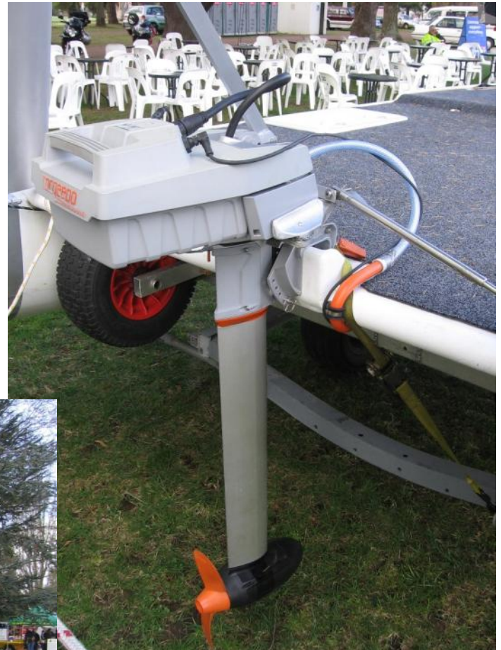
'Moondog' Solar powered catamaran with Torqueedo electric outboard
