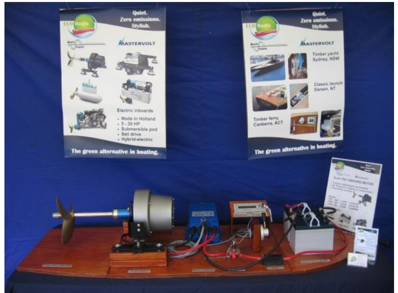
Inboard electric motor display
