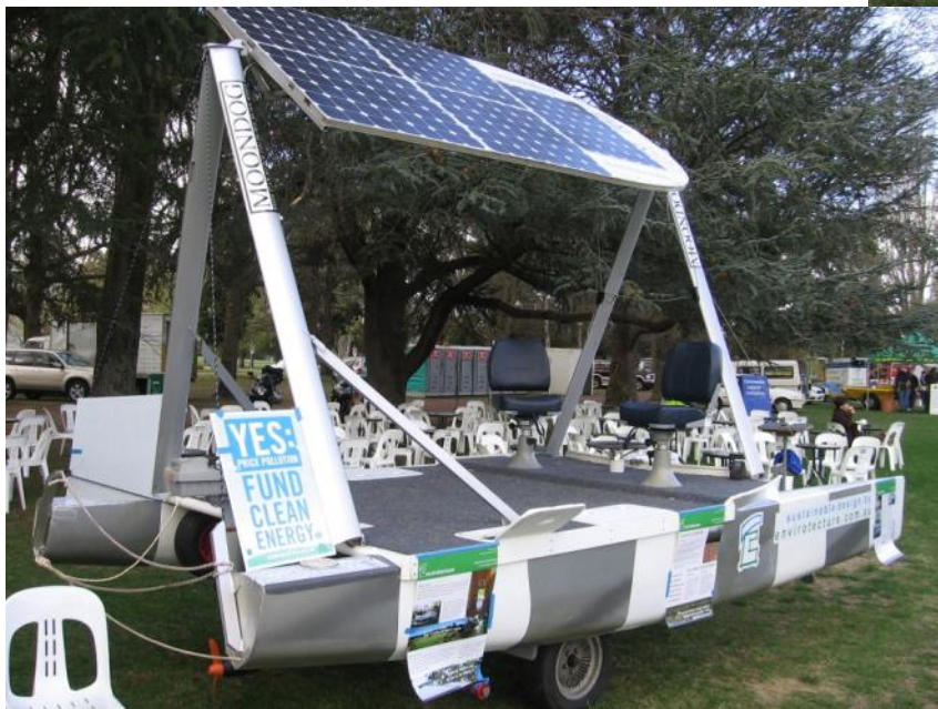
'Moondog' Solar powered catamaran with Torqueedo electric outboard
